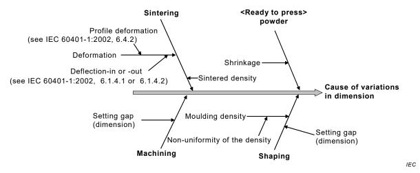
Figure 1 - Cause-and-effect diagram of variations in dimension
